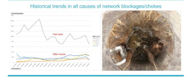
Figure 2-7 Historical trends in all causes of network blockages/chokes and a typical image
