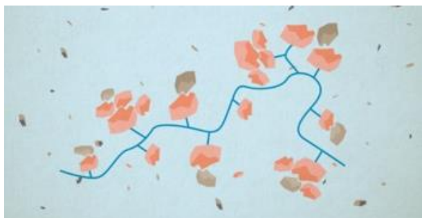
Polymer chain sticking particles together, forming flocs.
